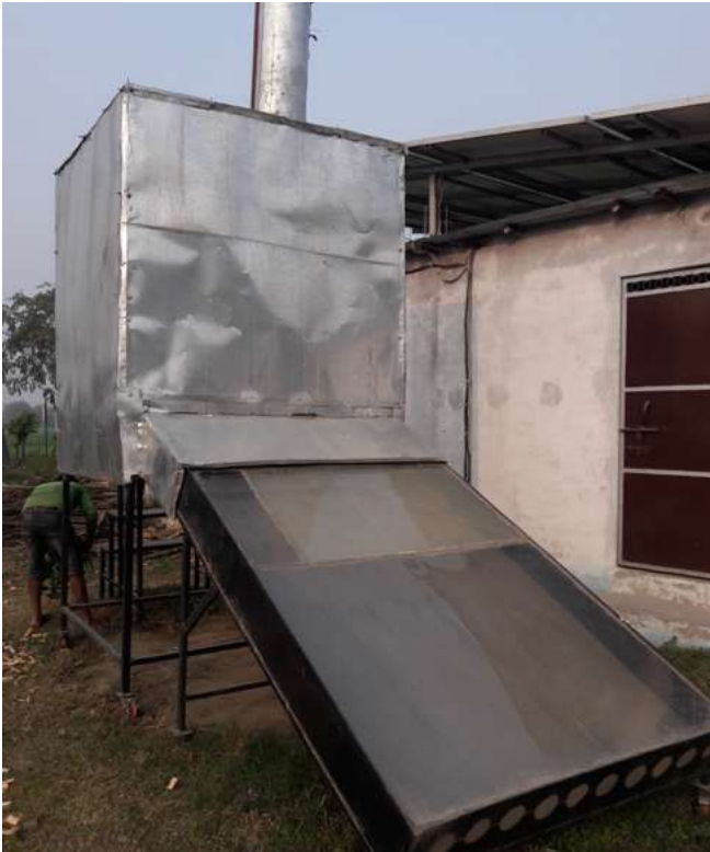
In-house made solar chimney dryer with trays to dry different vegetables and spices at the same time (Bihar 2018)
