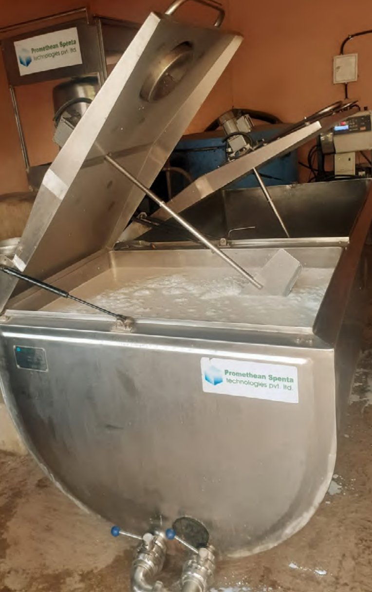
1,000 litre Split Tank Bulk Milk Cooler (chilling cow and buffalo milk separately) installed for ITC dairy in Munger (Bihar, 2017)
