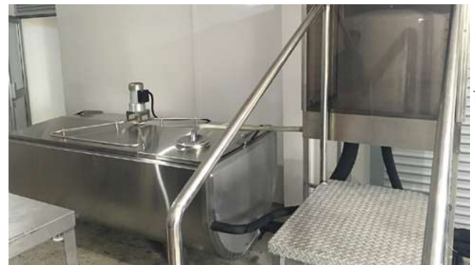
1,000 litre Rapid Milk Chiller installed near Colombo (Sri Lanka, 2015)
