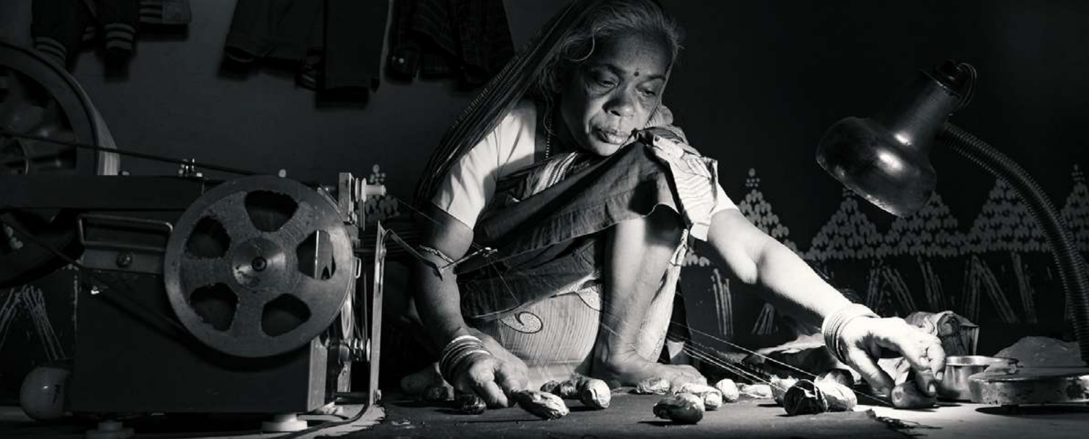
The woman switched from arduous thigh reeling method to using solar powered buniyaad machine for silk reeling. (Odisha 2018)
