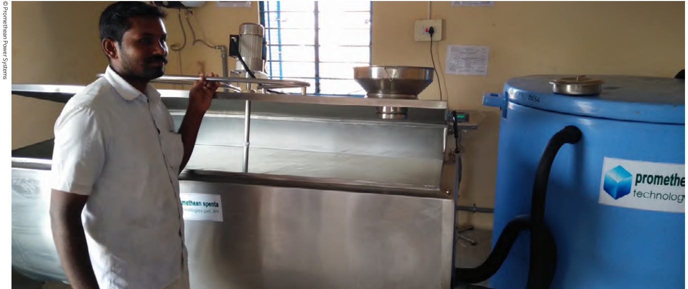
1,000 litre Bulk Milk Cooler installed in Salem (Tamil Nadu, 2016)
