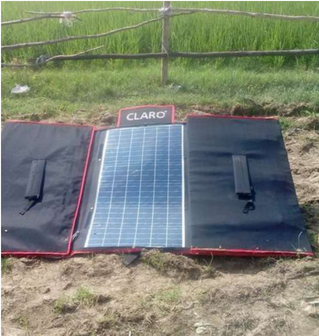
The lightweight solar panels fold into an easy to haul backpack. (Bihar 2018)
