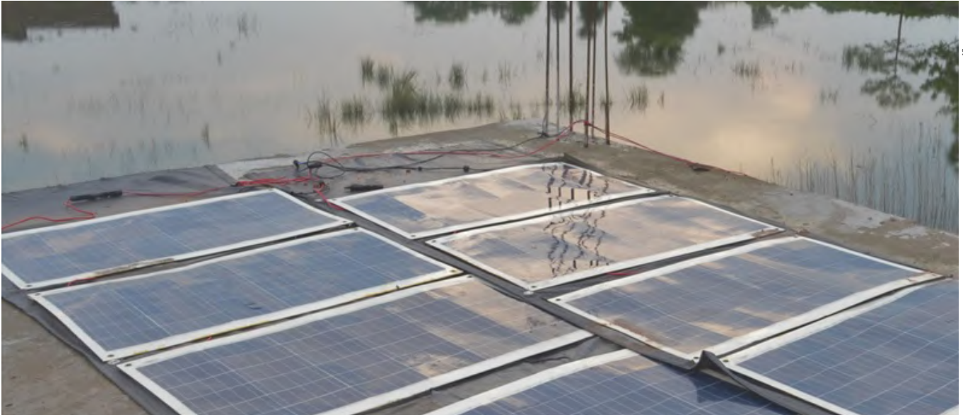
A lightweight foldable portable solar pump for the smallholder farmer
