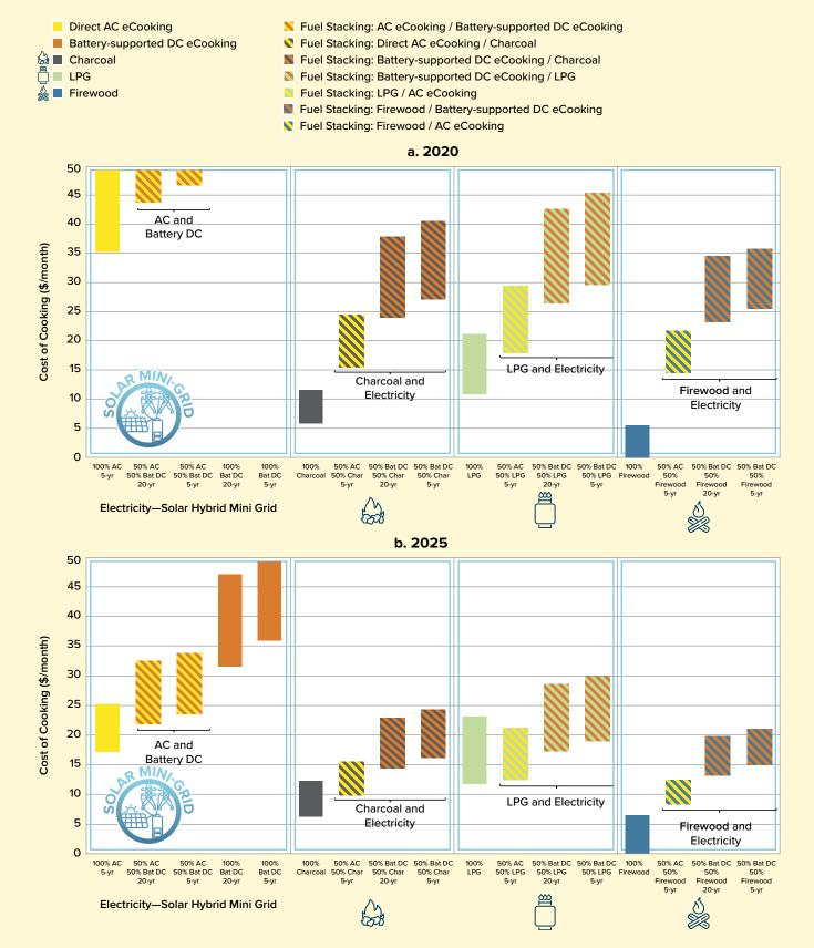
Note: ESMAP's (2019a) typical solar hybrid mini grid tariffs of \$0.55-\$0.85/kWh from 2018 are assumed applicable in 2020; its optimized solar hybrid mini grid tariffs of \$0.25-\$0.38/kWh are applied in 2025. Where applicable, batteries are LiFePO4 sized for 50 percent (0.97kWh) or 100 percent (2.98kWh) of daily cooking load.
