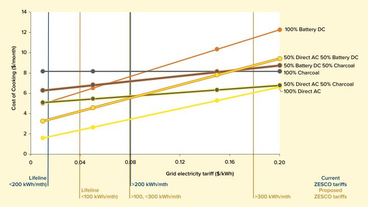
Note: Where applicable, batteries are LiFePO4 sized for 50 percent (0.42kWh) or 100 percent (1.3kWh) of daily cooking load. All scenarios are modelled with a 20-year financing horizon.
