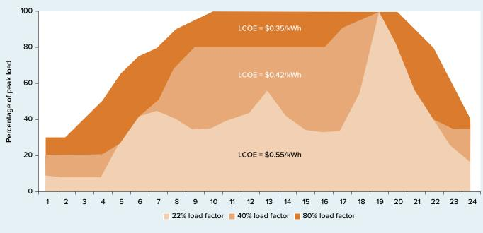
FIGURE 3.15 Effect of increasing load factor on levelized cost of electricity of power-limited mini grids
