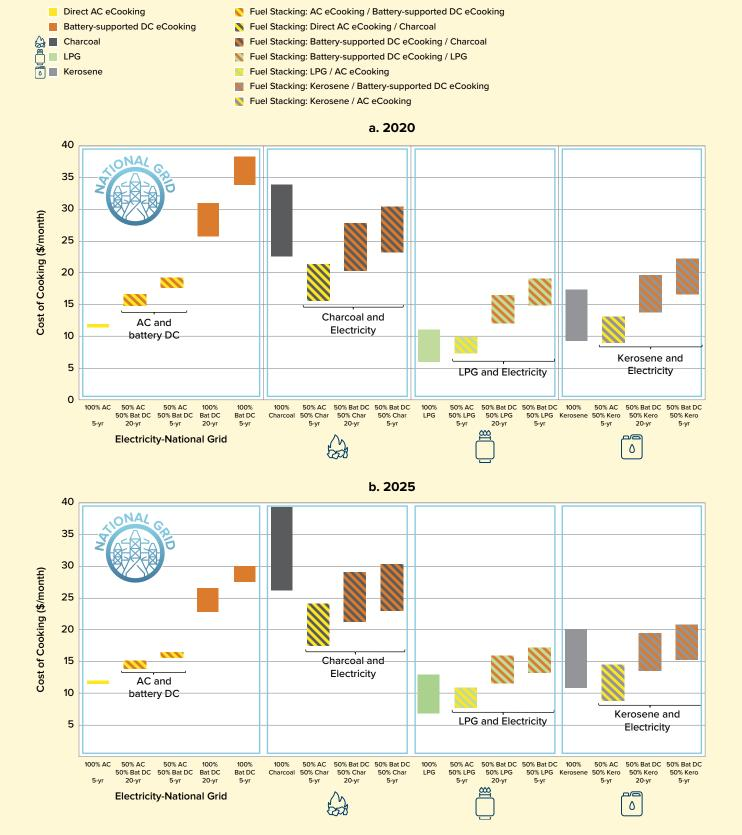
Note: Grid tariff of \$0.17/kWh corresponds to price of the first 100kWh/month from KPLC in 2019. Where applicable, batteries are LiFePO4 sized for 50 percent (0.93kWh) or 100 percent (2.78kWh) of daily cooking load.
