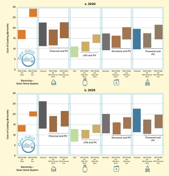
Note: Where applicable, batteries are LiFePO4 sized for 50 percent of the menu on a DC PV-powered battery-supported EPC (0.74kWh capacity, 220Wpeak PV) and stacking with charcoal, LPG, or kerosene, or cooking 100 percent of the menu (2.2kWh battery and 630W<sub>neak</sub> PV.)
