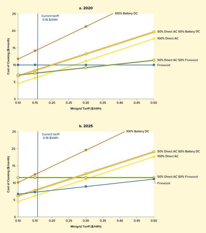
Note: Figure shows when each eCooking scenario could become cost-effective. It therefore uses the upper bound of the traditional fuel price ranges and the lowerbound assumptions for eCooking costs, with the 20-year financing model. Where applicable, batteries are LiFePO4 sized for 50 percent (0.52kWh) or 100 percent (1.56kWh) of daily cooking load.
