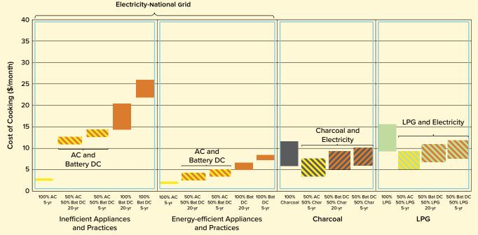
*Note:* Figure uses energy demand data from neighboring Tanzania, where cooking practices are similar, because insufficient cooking diary data were available for LPG in Zambia. Where applicable, batteries are LiFePO4 sized for 50 percent (0.42kWh) or 100 percent (1.46kWh) of daily cooking load. Grid tariff used is \$0.014/kWh, which corresponds to the 2019 price of the first 200kWh per month from ZESCO.
