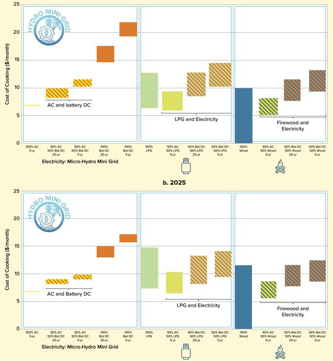
Note: Mini grid tariff is \$0.16/kWh. Where applicable, batteries are LiFePO4 sized for 50 percent (0.52kWh) or 100 percent (1.56kWh) of daily cooking load.
