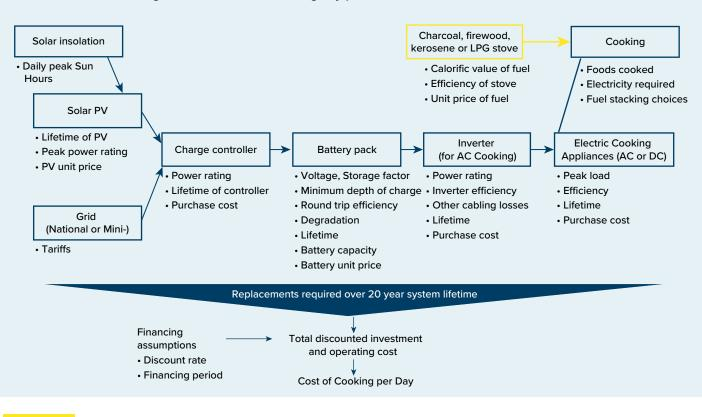
The energy needs for cooking define the requirements of one or more eCooking appliances and a matching inverter (if appliance uses AC electricity). The eCooking system is sized to meet a user-defined fraction of this total cooking demand, with the balance met from a specified traditional fuel.
