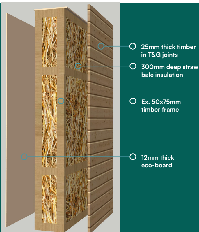
Figure 10. 3D visualisation of the key insulation materials
