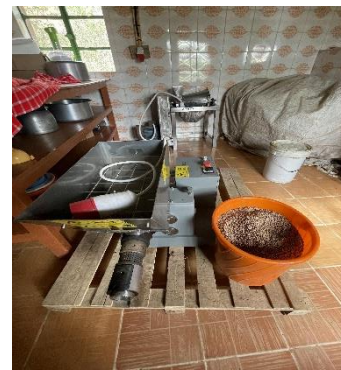
Image 20F: Cold pressed oil extractor imported from Germany
