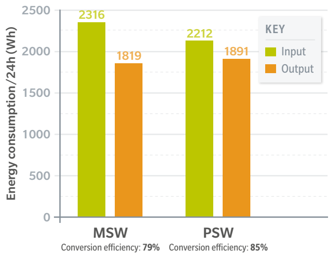
Figure 11: Energy consumption of all loads combined running on the MSW and PSW inverters, as input and output energy
