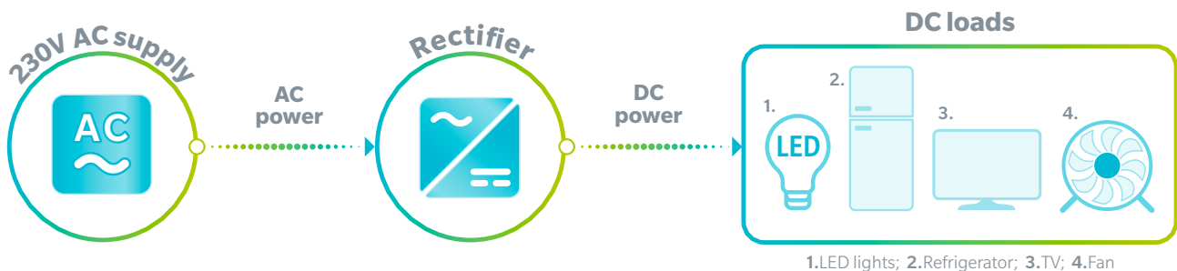
Figure 16: Schematic of multiple DC appliances operating on a 230V AC supply through a rectifier
