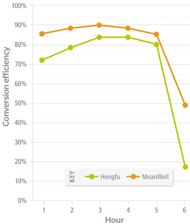
Figure 19: Conversion efficiency during each hour period on both the MeanWell (higher cost) and Hengfu (lower cost) rectifiers
