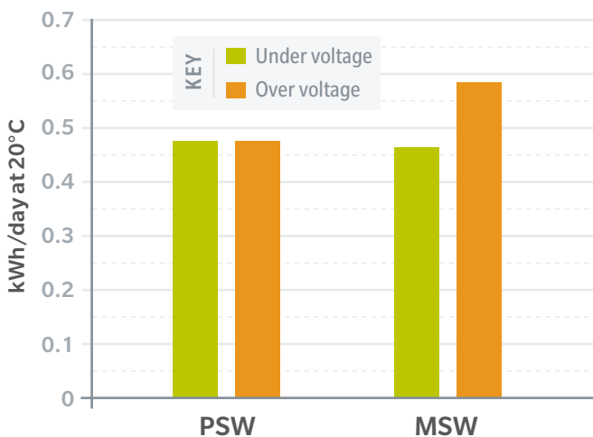
Figure 13 – Comparison of energy consumption of the Haier appliance operated on the PSW and MSW inverters in over- and under-voltage conditions
