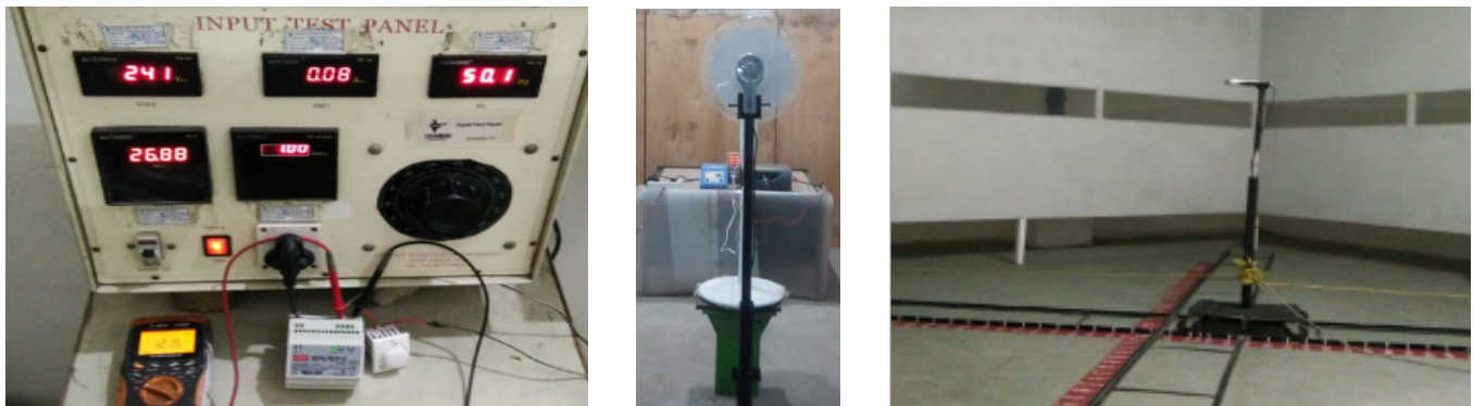
Figure 28 – Testing of DC fans with rectifiers
