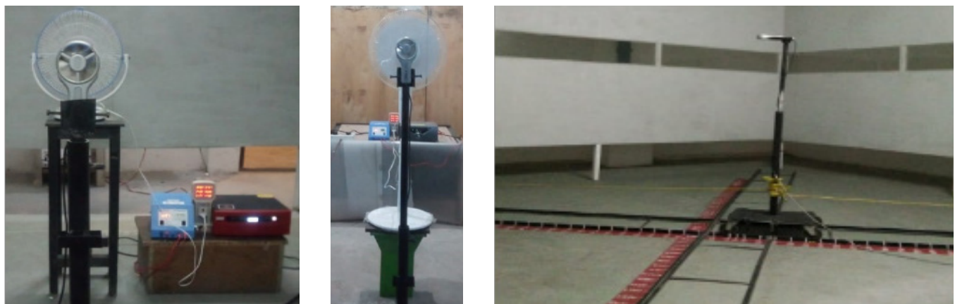
Figure 27 – Testing of the AC fans with inverters
