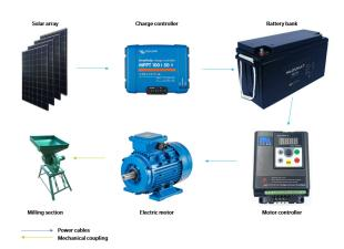
Figure 3: Layout of a direct-drive solar mil<sup>47</sup>
