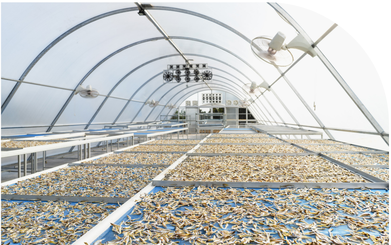
A greenhouse solar dryer with forced convection drying fish in Thailand Source: Venusvi, Getty Images, 2020,
