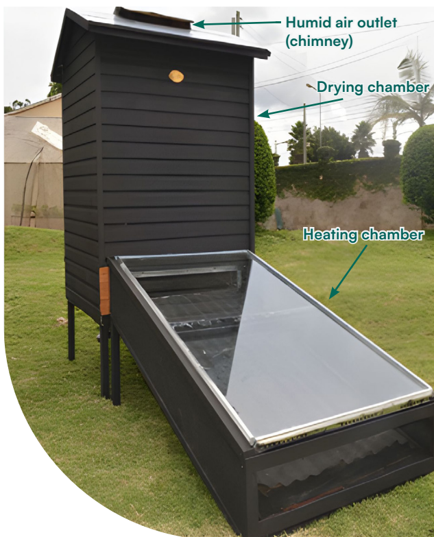
Figure 2: A cabinet solar dryer with natural convection Source: African Natural Products
