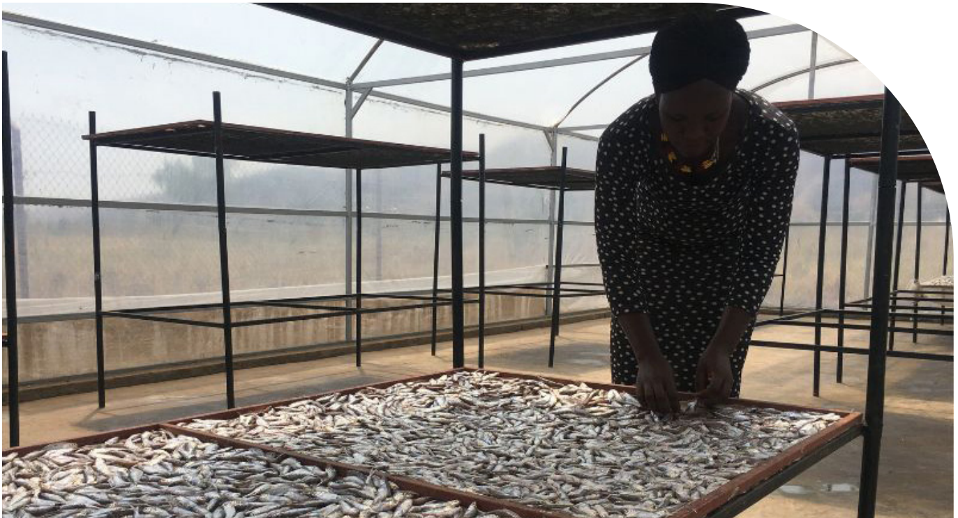
Figure 5: Silver cyprinids being dried in solar tent dryer installed under the NutriFish project in Kampala, Uganda Source: NutriFish project
