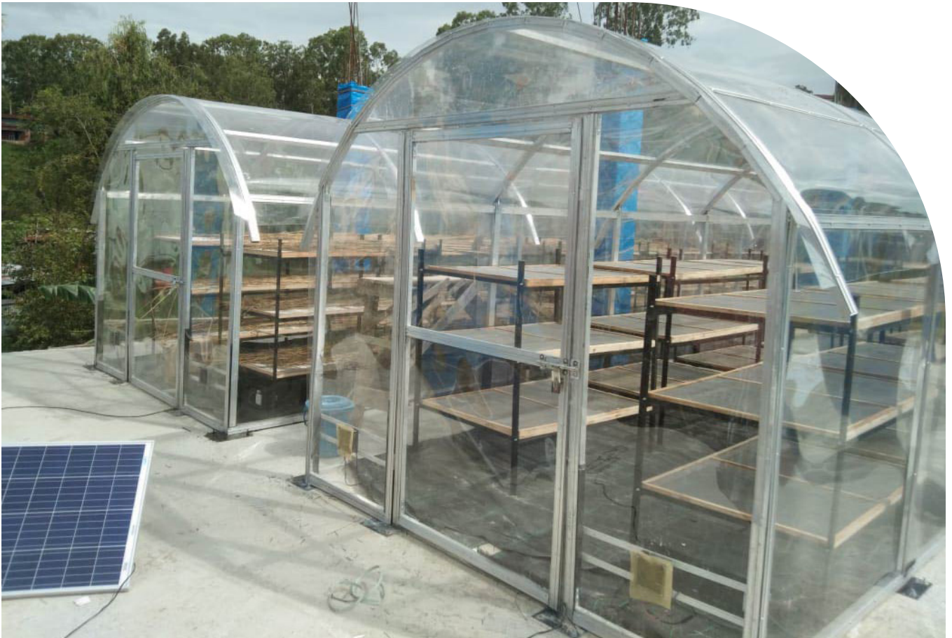
Figure 4: Greenhouse solar dryers constructed in India Source: Raheja Solar Food Processing
